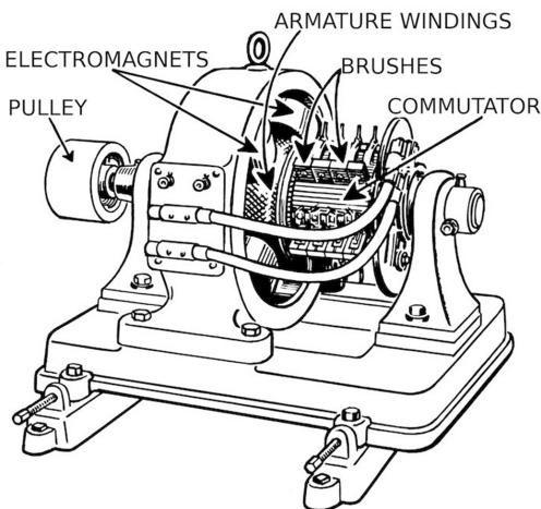
*Figure 6: The dynamo is a complicated machine producing electromagnetic fields and currents by mechanical motions. It must be constructed in an extremely special manner harnessing the physical laws.*
